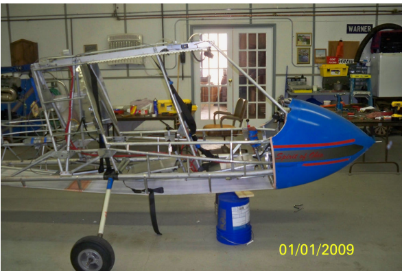
Stripped down for inspection
